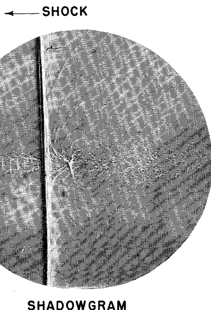
Fig. 2 Traveling shock-opposing axisymmetric jet interaction; S = 1.46 , x/d = 3.20 ; choked jet: p_{01j}/p_{1u} = 2.00 , d = \frac{1}{4} in., T_{01j} = 73^\circ\text{F}
